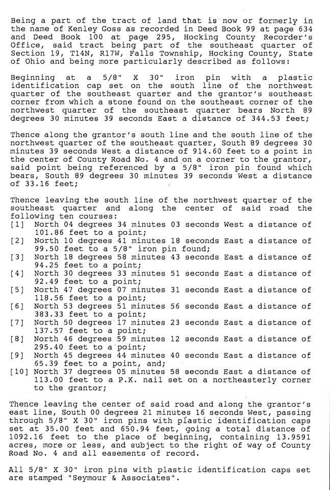
The bearings used in the above described tract were based on monuments found on the south line of the northwest quarter of the southeast quarter as bearing South 89 degrees 30 minutes 39 seconds West and are for the determination of angles only.
