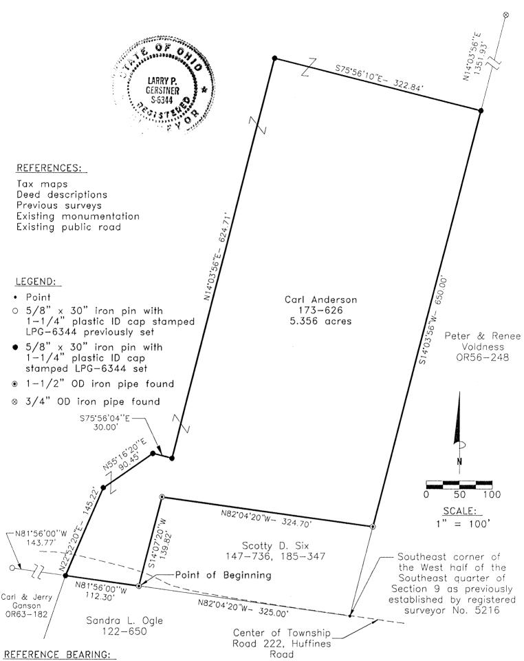
The East line of the West half of the Southeast quarter of Section 9 as South 14 degrees 03 minutes 56 seconds West. Bearings are based upon an assumed meridian and are to denote angles only. Approved - Mathematically
