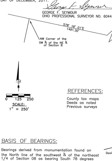
1/4 of Section 08 as bearing South 78 degrees 18 minutes 01 seconds East and are for the determination of angles only.
