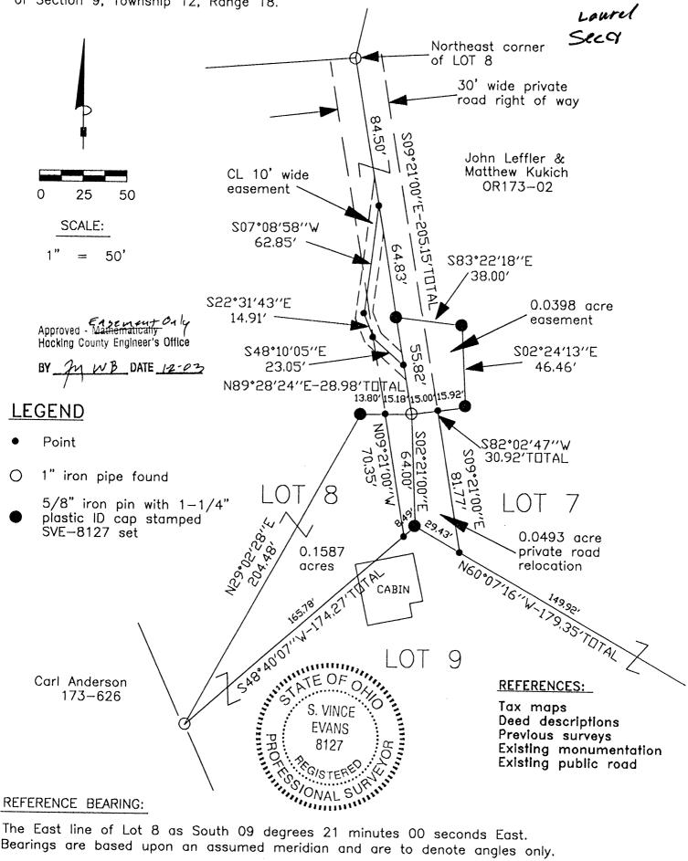
The East line of Lot 8 as South 09 degrees 21 minutes 00 seconds East. Bearings are based upon an assumed meridian and are to denote angles only.
