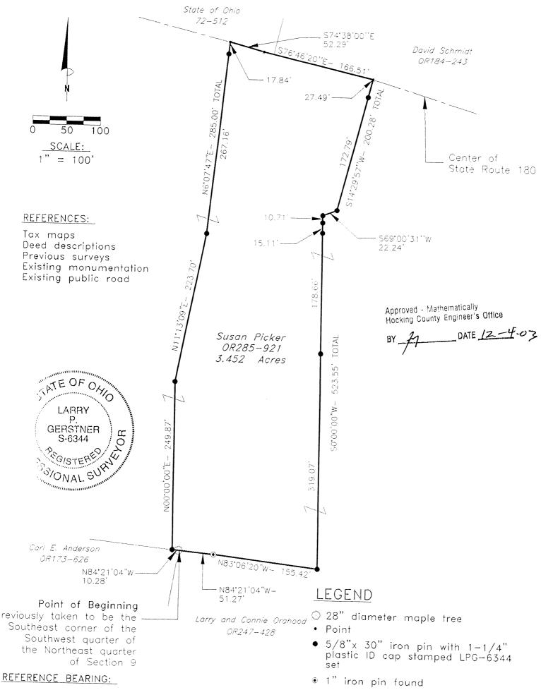
West line of a 11.99 acre survey as North 0 degrees 00 minutes 00 seconds East. Bearings are based upon an assumed meridian and are to denote angles only.
