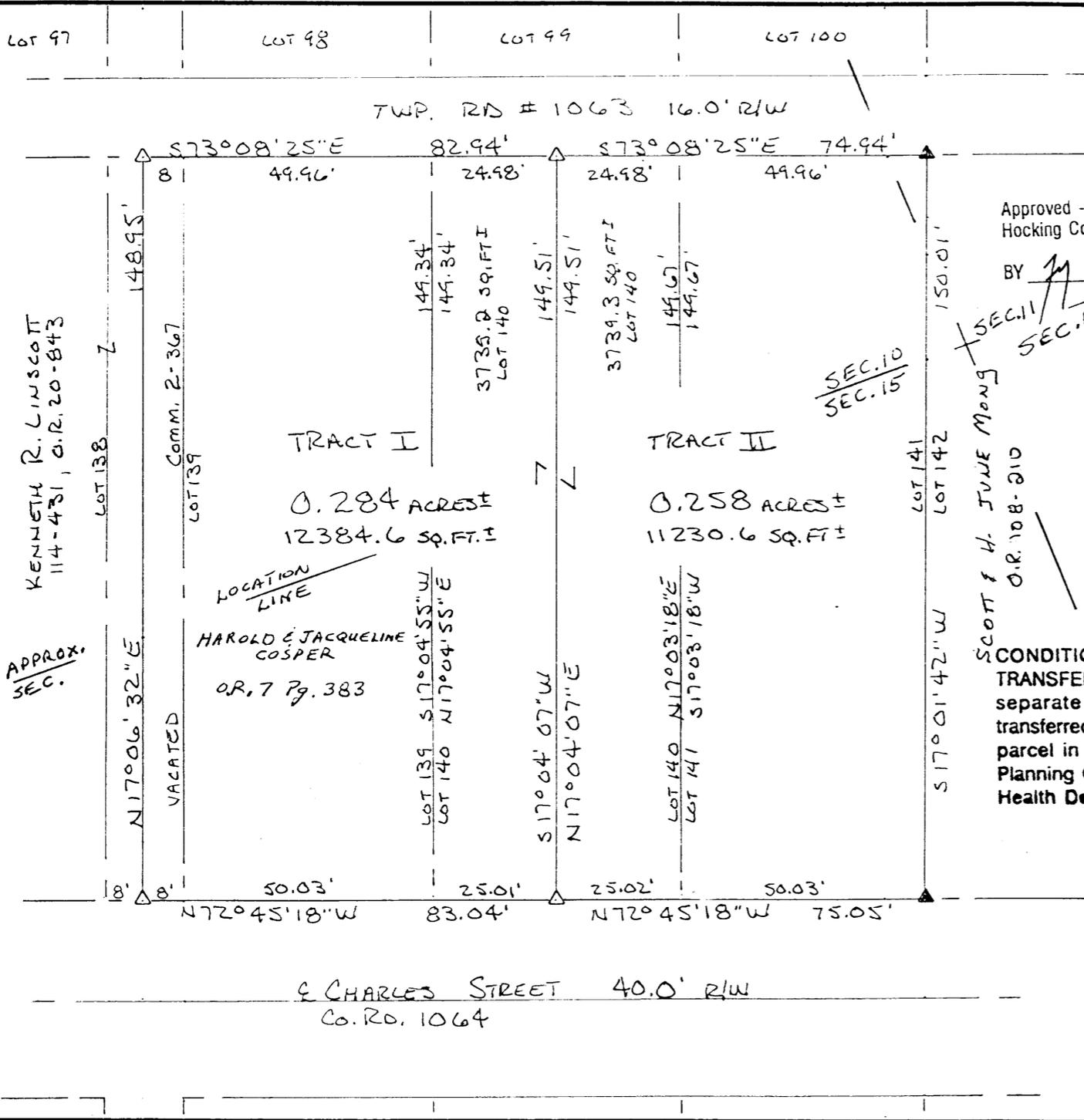
NOTE: BEARINGS WERE DERIVED FROM EASTLINE OF LOT 141 AS S17°01'42"W AND ARE FOR THE DETERMINATION OF ANGLES ONLY.
