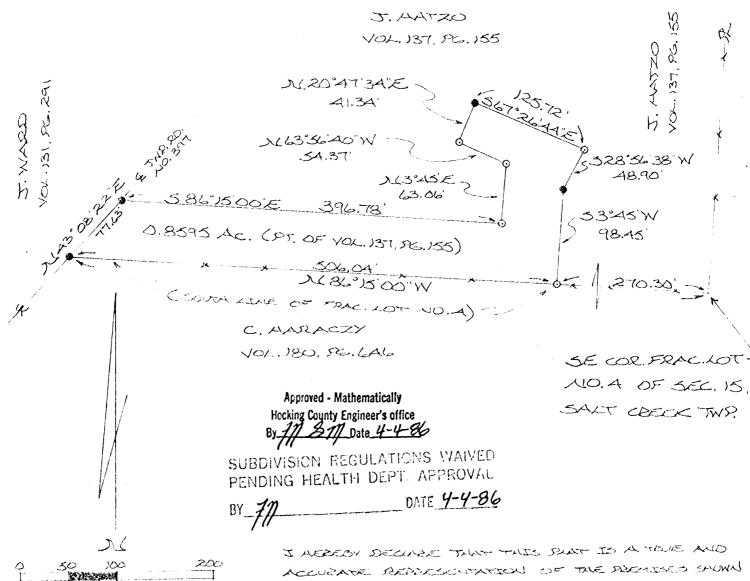
ARDEON AS DETERMENED BY AN ACTUAL SURVEY MADE SCALE:)"=100" UNDER AU DIDECT SUPERVISION ON THE LATE DAY 0 = 1/2" IRON PIN(S) W/ID CAP OF MARK, 1986. = SPICE NAIL (E) \* \* = EXISTING FERKE
