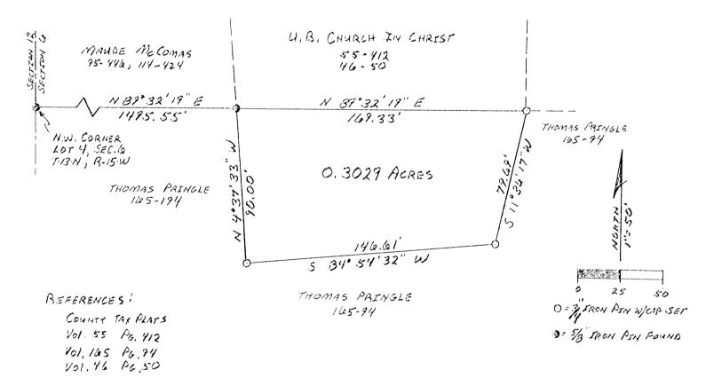
HOTE: BEARINGS DERIVED FROM PREVIOUS SURVEY AND ARE FOR DETERMINATION OF ANGLES ONLY.
